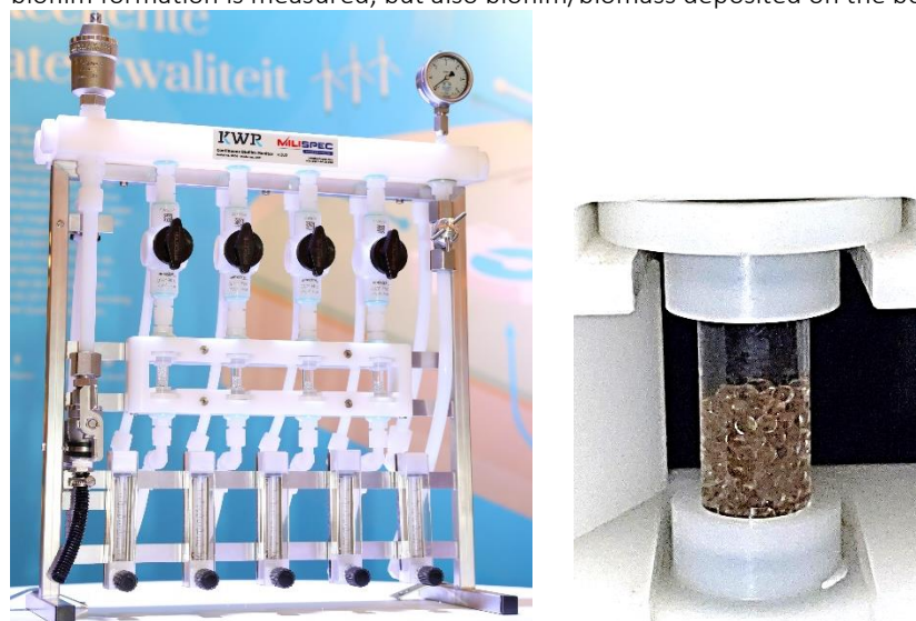
Figure 2-6. Continuous Biofilm Monitor (CBM) of Milispec (left) and a close-up of a cuvette with glass pearls (right)
