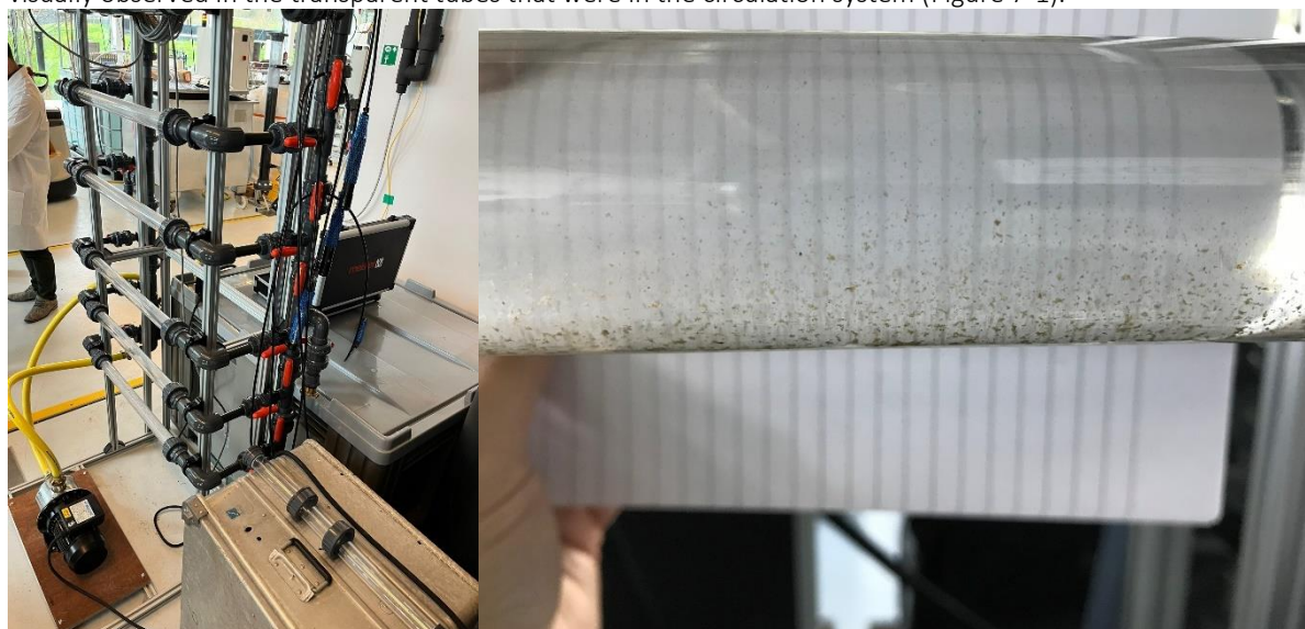
Figure 7-1: transparent tube for observation of biofilm growth.
