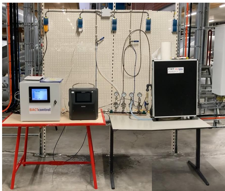
Figure 6-3. Installation of BACTcontrol, BactoSense and Milispec-CBM at production location Spannenburg, Vitens. The splitting station was placed between the BactoSense and the CBM.
