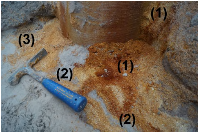
Garzweiler (1) Incrustations at screen (2) Aquifer sand pockets in gravel pack (3) Uneven incrustation distribution in gravel pack Photo: Houben
